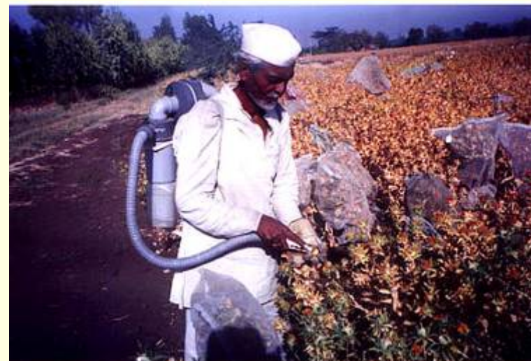
Solar powered safflower petal collector
