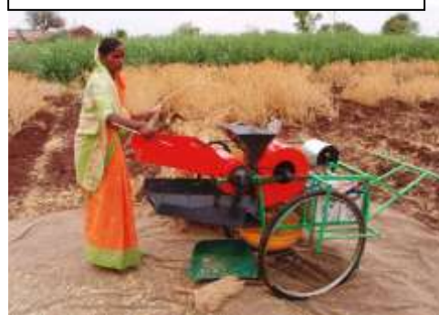
Battery powered safflower thresher
