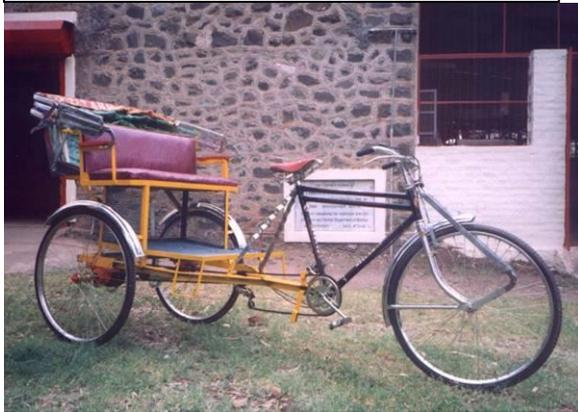
We then designed a [lightweight and easy-to-drive rickshaw](#) and tested it on Phaltan roads. However, converting this improved rickshaw into an electric-powered one proved to be quite difficult, since in those days (mid 1990s) small, high-torque permanent magnet D.C. (PMDC) motors and controllers were not
