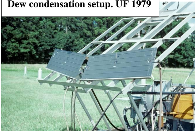
Dew condensation setup. UF 1979
