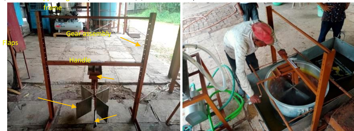
Figure 11: Semi-mechanical cooling device. Left: while not in operation; right: during syrup-making session.
