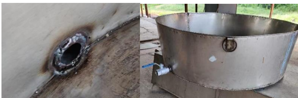
Figure 45: Development of the evaporation pan. Left: drain near the bottom; right: zoomed out view of the pan.
