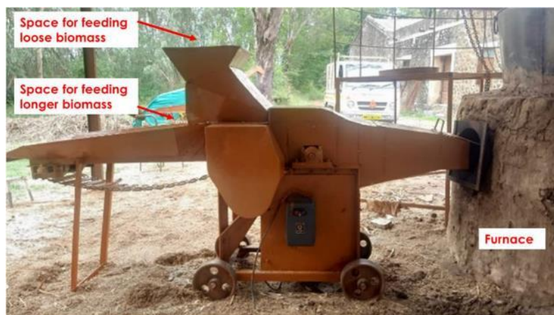
Figure 9: Shredder cum feeder cum air-blower designed in-house.
