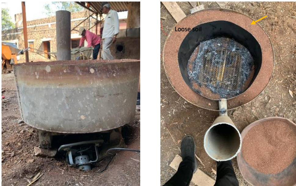
Figure 152: Design 1 for pan sealing using loose soil.
