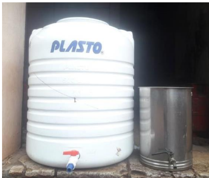
Figure 36: Left: new 500 L plastic settling tank; right: previously used 60 L stainless steel settling tank.
