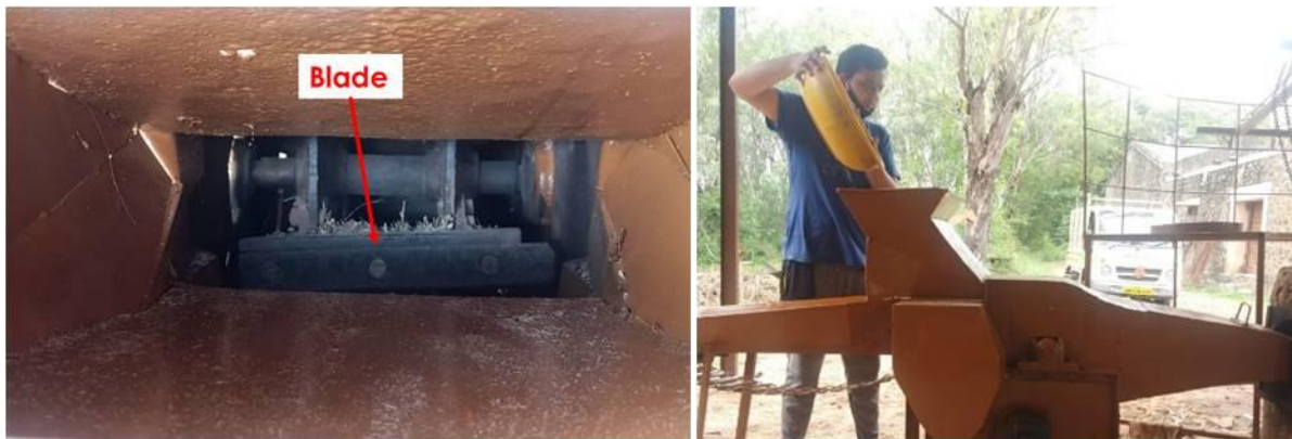
Figure 131: Modification in the shredder machine to feed loose biomass.
