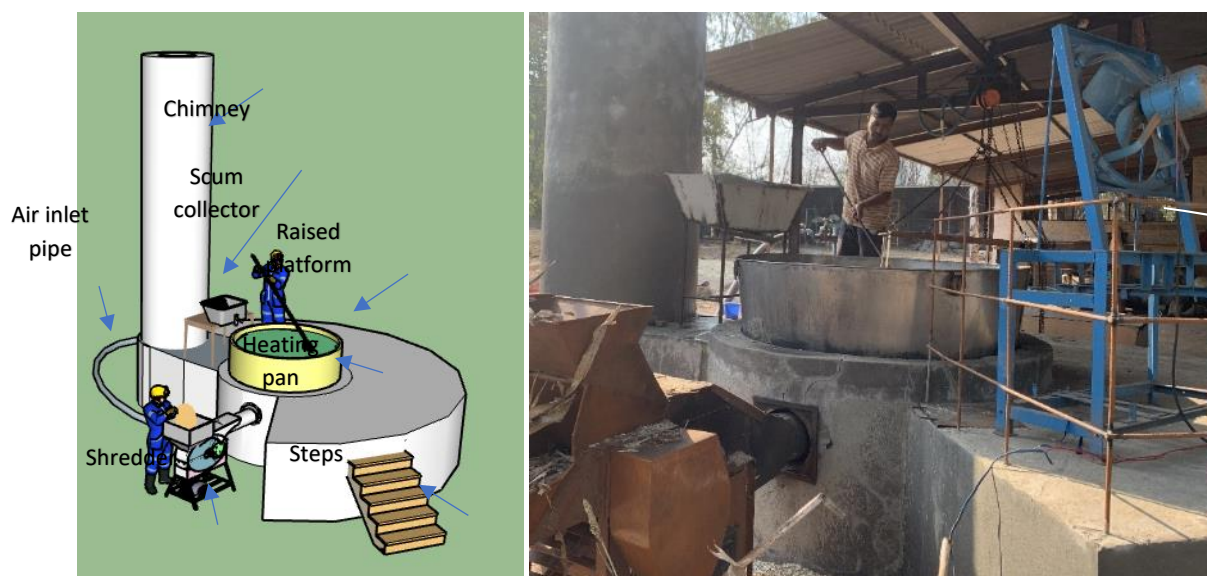
Figure 72: Left: A schematic of the new furnace; right: actual photo.
