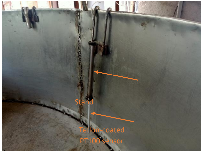
Figure 54: Teflon-coated PT100 sensor used for measuring juice temperature.
