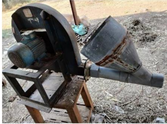
Figure 128: Fuel-feeding using blower and hopper.
