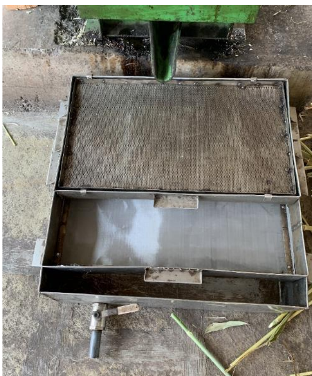
Figure 34: New stainless-steel juice filtration unit. In this picture, the first three filters of this unit of sizes 2500, 750 and 250 microns, respectively, are seen. The fourth mesh of 100-microns size is used while transferring the juice from settling tank to heating pan.
