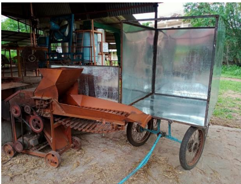
Figure 64: Cart for storing bagasse and leaves during feeding.
