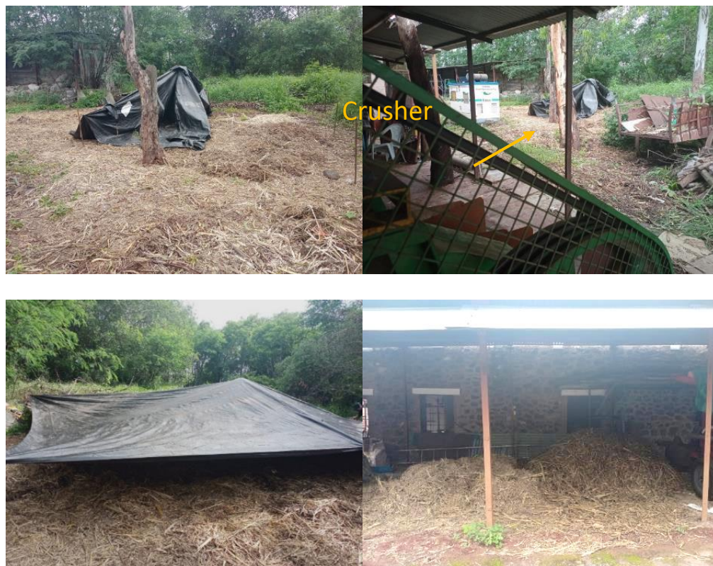
Figure 32: Bagasse drying system. Top-left: bagasse drying area; top-right: bagasse drying area as viewed from crusher; bottom-left: tent for protecting bagasse from rain while allowing air passage; bottom-right: shed for dried bagasse and leaves.
