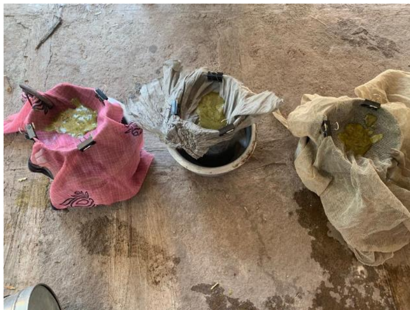
Figure 118: Immediately after the first scum layer removal. At this point, it is difficult to tell the three meshes apart. The difference in their performance becomes clear over a longer time period.
