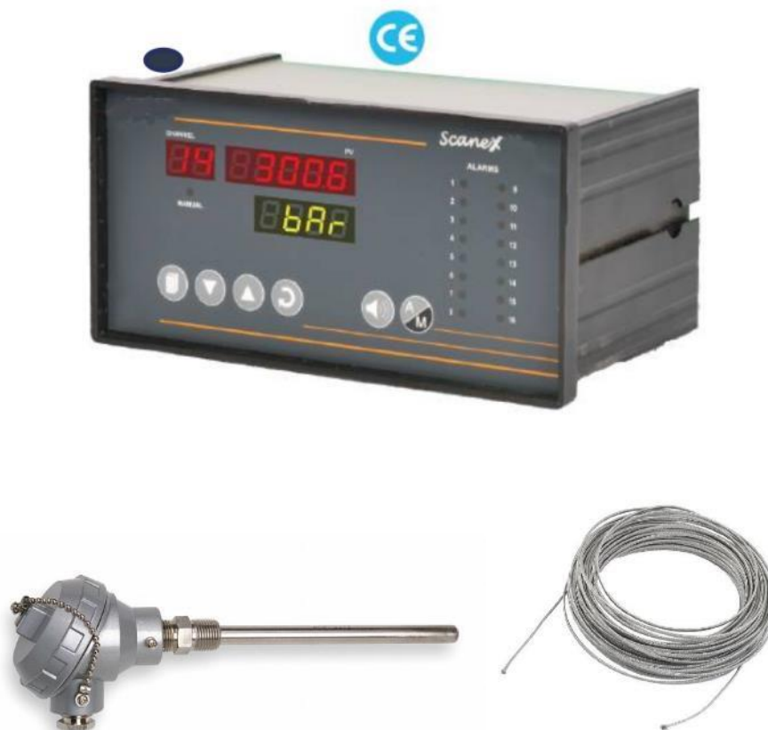
Figure 53: Top: eight channel digital scanner (courtesy: Protek Instruments, Pune); bottom-left: K-type thermocouple probe; bottom-right: K-type thermocouple wire.
