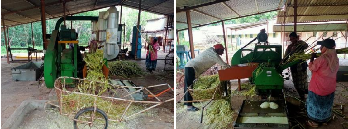
Figure 4: New three-roller crusher. Left: back view; right: side view.
