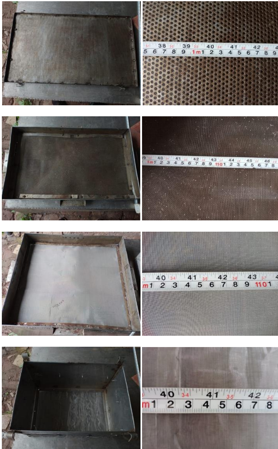
Figure 105: Four filters from coarsest (top-row) to finest (bottom-row). In the right column, close-ups with a scale alongside are presented.
