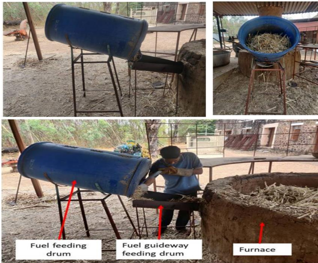
Figure 127: Fuel-feeding using drum and guideway.
