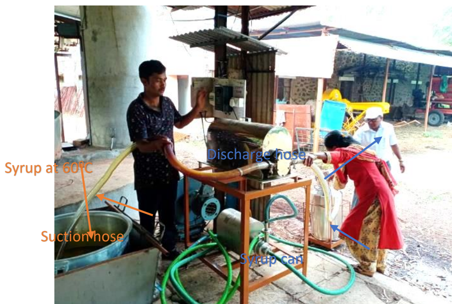
Figure 85: Pumping of syrup from cooling pan to storage can.
