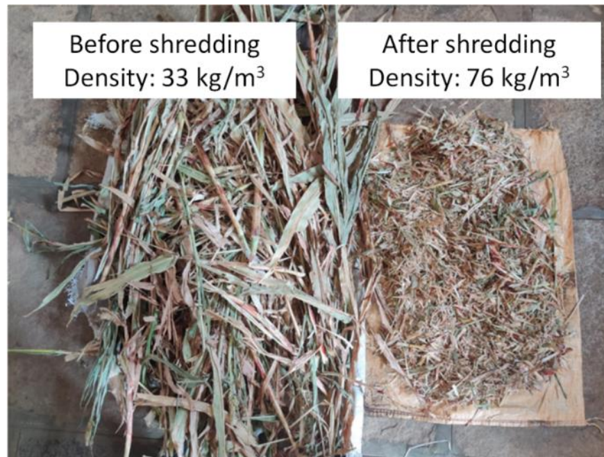
Figure 138: SS leaves. Left: loose; right: shredded.
