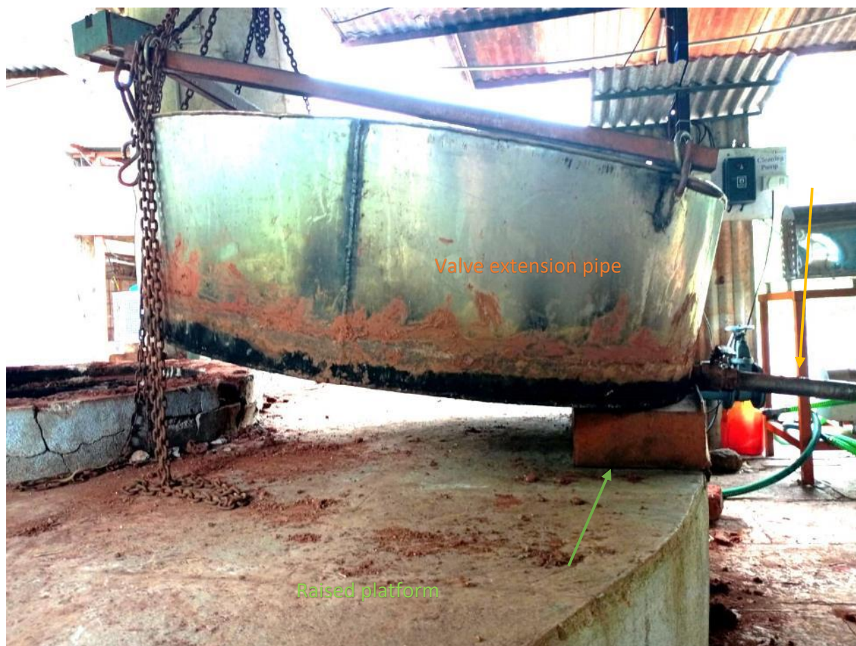
Figure 75: A raised platform was constructed for convenient pan-tilting.
