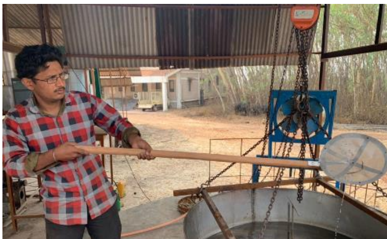
Figure 44: Bigger scum removal ladles. Top: close-up view; bottom: while in operation.
