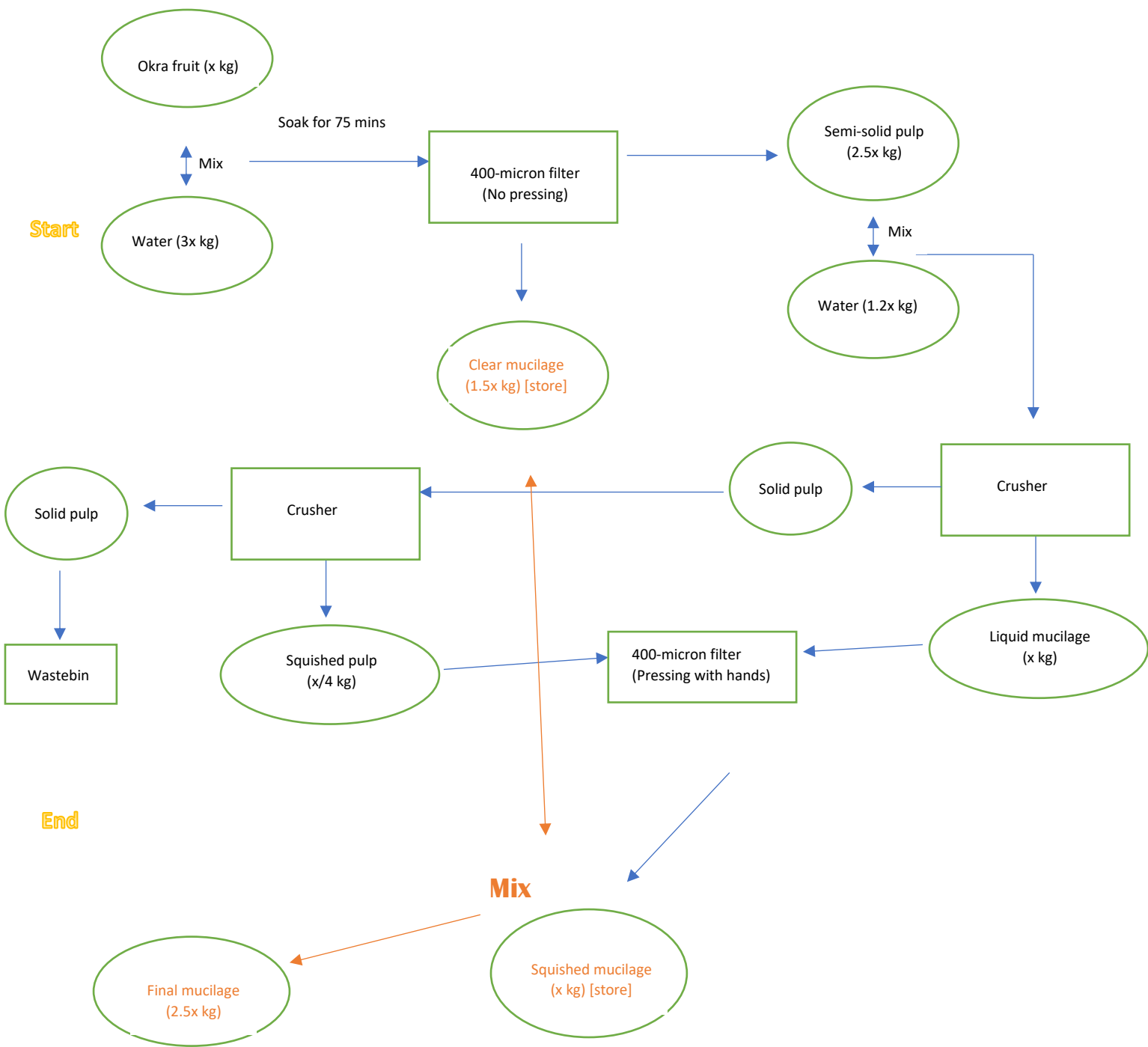
Figure 116: Mucilage preparation methodology.
