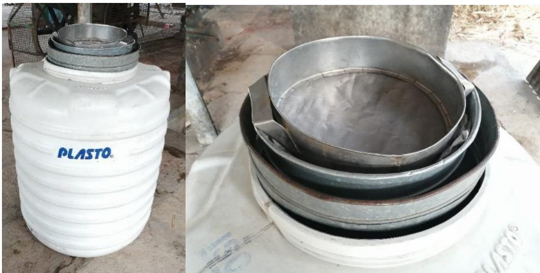
Figure 33: Smaller circular meshes used for juice filtration earlier.
