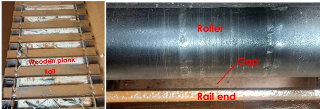
Figure 130: Filling up of gaps in the feeder of the shredding machine.
