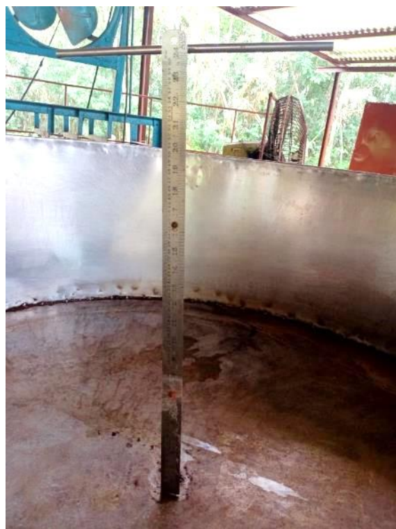
Figure 47: Stainless-steel scale for measuring juice level in heating pan.
