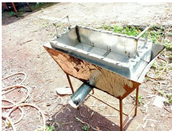
Figure 43: Scum collector. Top-row: usage during syrup-making; bottom: while not in use.
