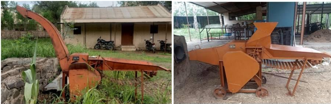
Figure 129: Left: chute of the old shredder machine; right: modified chute.
