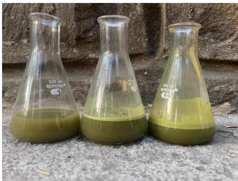
Figure 120: Filtered juice from the three meshes. The juice obtained from the stainless-steel mesh (left) is clear and contains no foam. The juice becomes less clear and foamier as we move rightwards (middle: saree, right: mosquito net). Note that in the scum collector, this clear juice is drained back to the heating pan.
