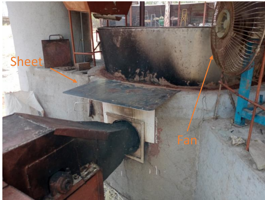
Figure 73: Fan for blowing away ash particles away from the juice and sheet to block them.
