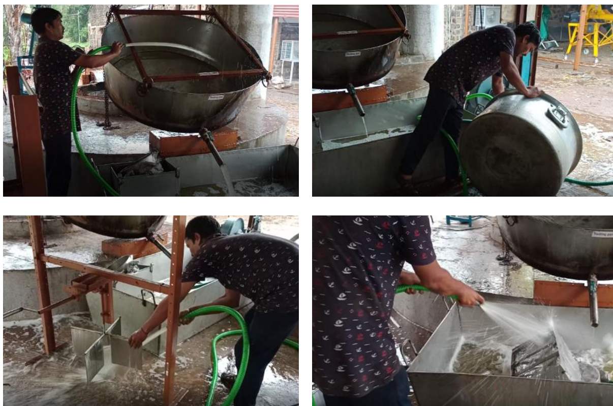
Figure 86: Pressure washing using the cleaning pump. Top-left: heating pan; top-right: cooling pan; bottom-left: semi-mechanical cooling machine; bottom-right: juice cum syrup filter.
