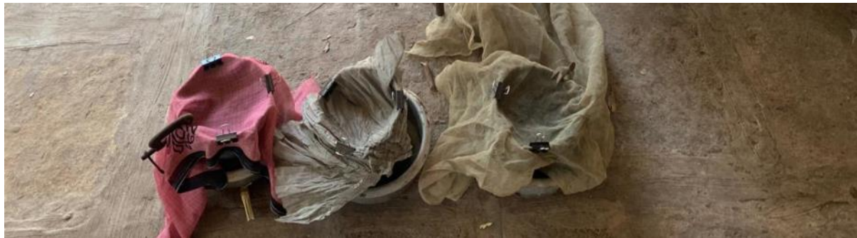
Figure 117: Meshes considered for scum collector. Left: saree; middle: stainless-steel mesh; right: mosquito net.
