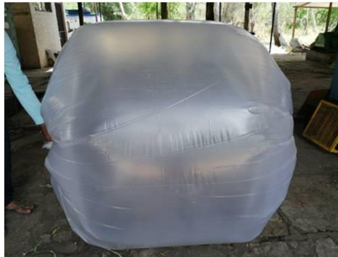
Figure 154: Filled plastic bag used for blower calibration.
