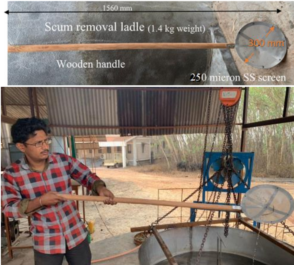
Figure 7: Bigger scum removal ladle. Top: close-up view; bottom: while in operation.
