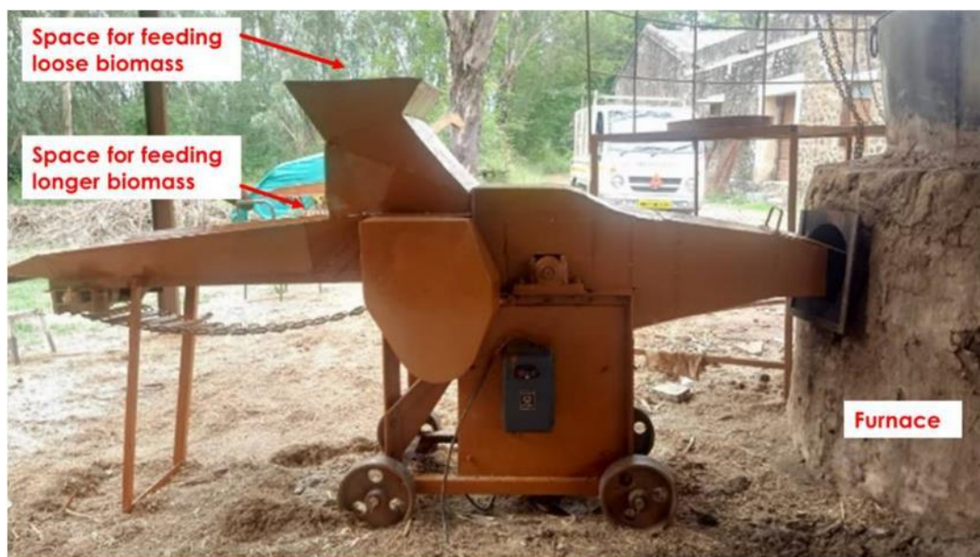
Figure 49: Fuel-feeding strategies tried. Top-left: a drum and guideway, top-right: a blower and a hopper, bottom: modified shredder (modified shredder was finalized).
