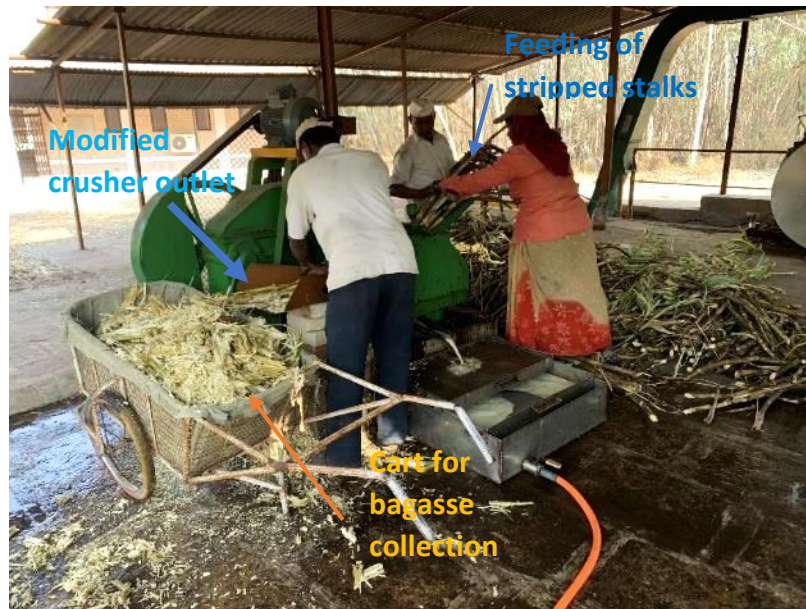
Figure 31: New method of wet bagasse collection.
