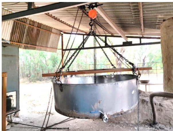
Figure 8: Block-and-tackle mechanism for lifting evaporation pan.
