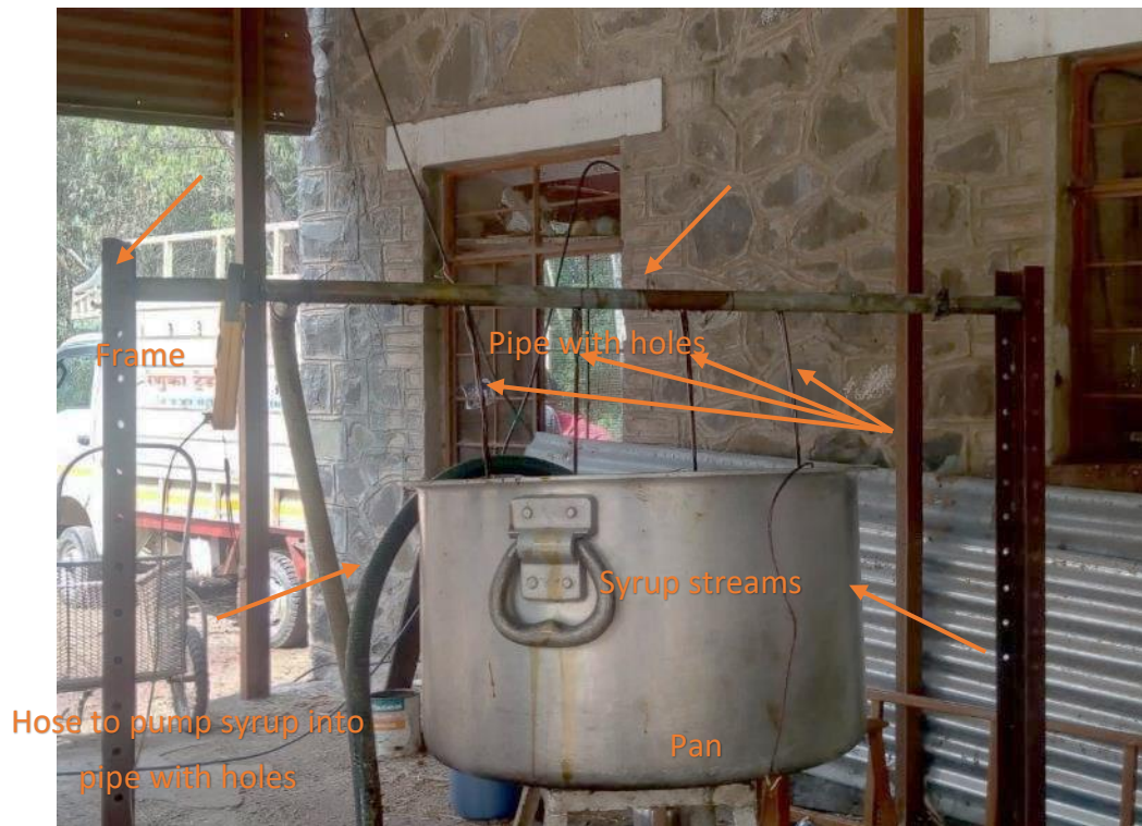
Figure 77: Preliminary cooling device that used cooling by natural convection through air.
