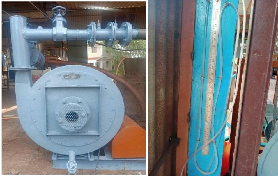
Figure 69: Left: blower for supplying air to the furnace; right: orifice meter.
