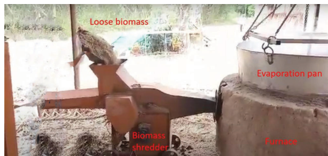
Figure 4. Fuel feeding into the furnace.
