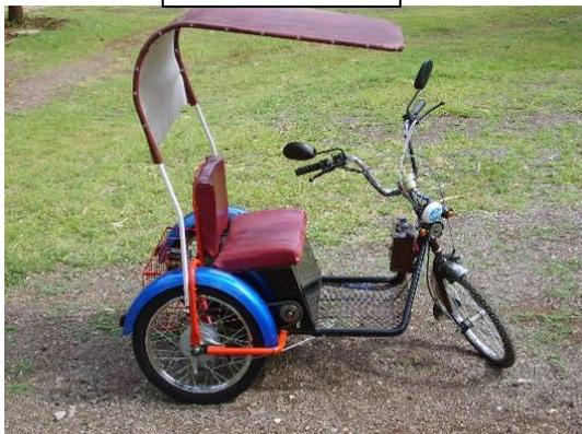
Because of our experience with designing electric cycle rickshaws we designed [two rickshaws for handicapped persons](#). One was a Motor Assisted NARI Handicapped Rickshaw (MANHARA), and the other was a completely automated rickshaw called an electric trike. Both have been given to few handicapped persons. An [excellent video on trike and MANHARA was shot in 2009](#).
