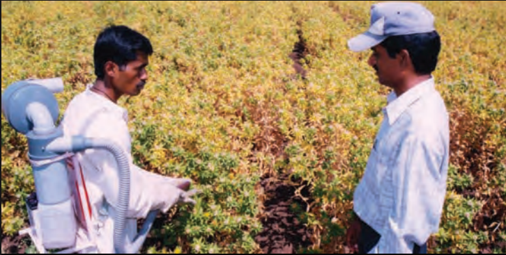
Battery powered safflower petal collector developed by NARI in use, 2005
