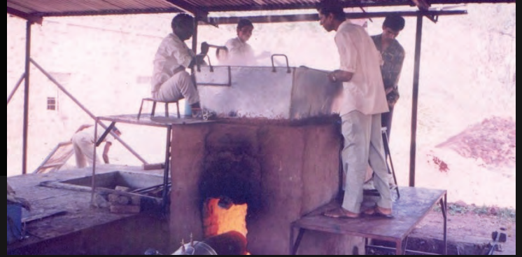
Sweet sorghum syrup preparation using gasifier, 1996
