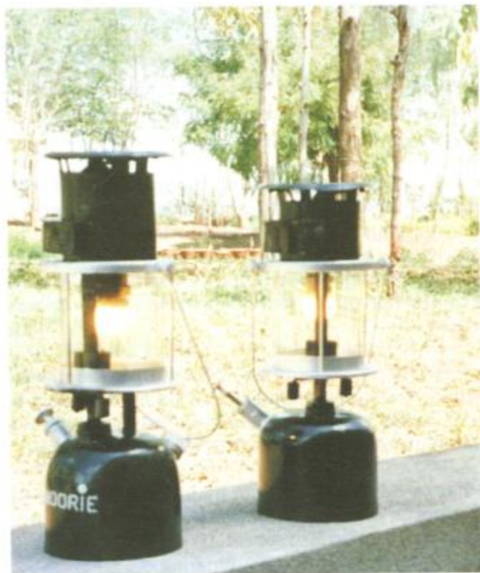
Alcohol lanterns which produce light equivalent to that from a 100-W electric bulb.
