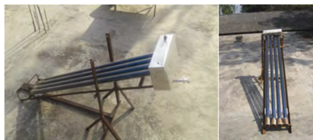
Figure 1. Four-tube solar water purifier.
