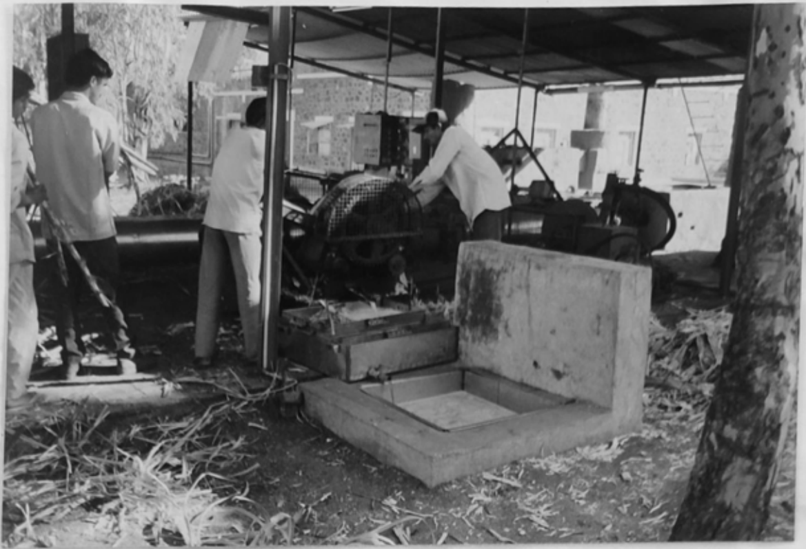
Crusher and Juice Clarification System
